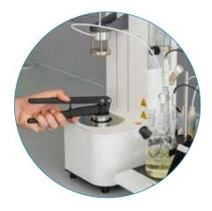
Why semi-automatic? The user places the sample in the oven with the crimper and starts the method on the titrator or (optionally) on the TitriSoft software. Apart from entering the sample name and, if necessary, the initial weight, this is all that needs to be done in the next few minutes-
